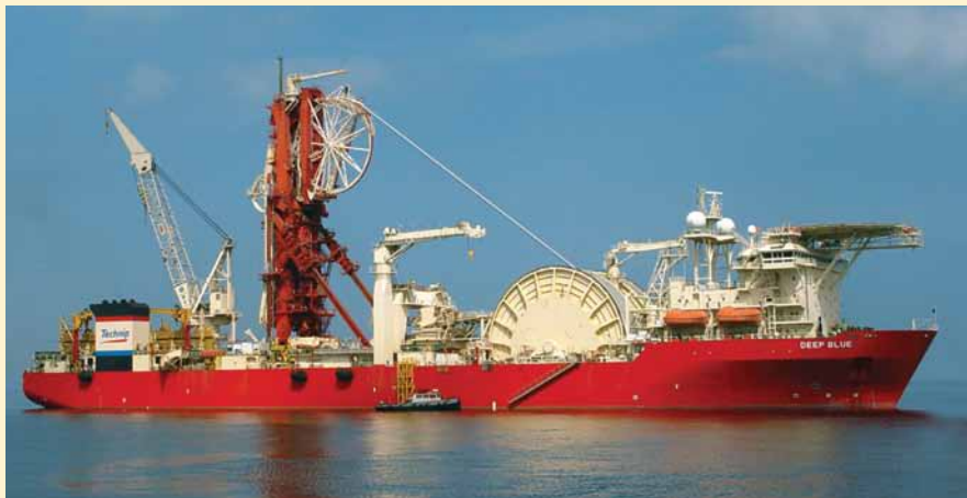
Technip used its high-technology Deep Blue vessel to lay pipelines and risers for the Shell Perdido project
