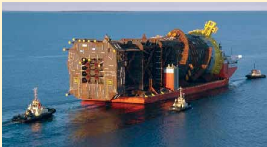
Perdido Spar as it is being transported to the final outfitting yard in the Gulf of Mexico.
