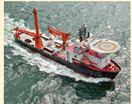
Cranes aboard the 430-foot DP-3 HOS Iron Horse MPSV can lift up to 400 tons of cargo.
