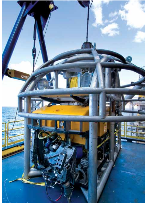
Because of the extreme water depth, remotely-operated vehicles (ROVs) like this one were used to complete much of the subsea work.
