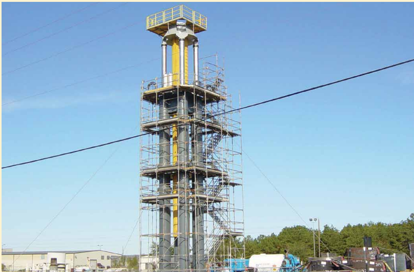
An assembled Perdido riser tensioner during factory acceptance testing, partially stroked out, but without the accumulators.
