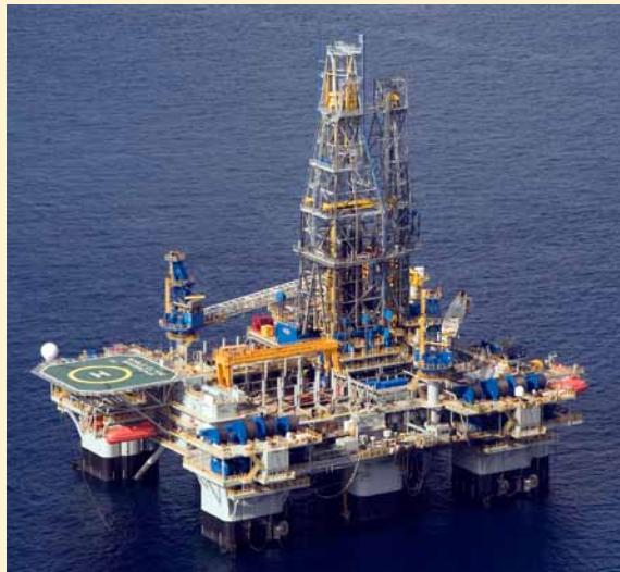
The Noble Clyde Boudreaux batch drilled 23 wells for Shell's Perdido development project while moored in water depths up to 9,000 ft.
