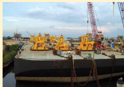
The PLETs for Perdido being loaded to barge at Bayou's waterfront facility.
